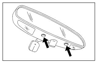
The mirror may also be equipped with reading lamps.
